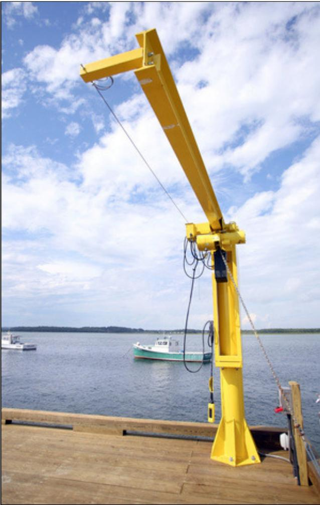
The new municipal pier at Pine Point in Scarborough has two hydraulic hoists that can help load gear and bait directly from trucks to boats, saving time and effort.
